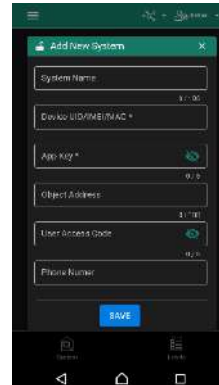
5. GTCOM2 sends a message with the IMEI 6. Enter the IMEI and App Key (Default 123456), Enter User access code (Default 123456)
